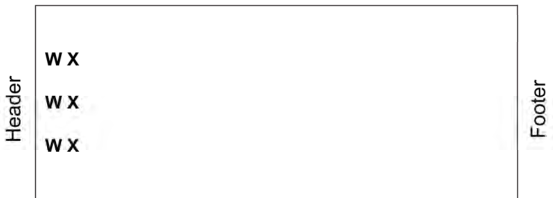
FIGURE 22 : SECURING THE HEADER END OF ATTIC LADDER
